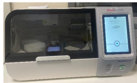
The Kingfisher robot for DNA extraction
