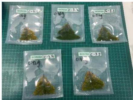
Buffer added into the extraction bags ready for homogenisation
