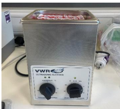
The sonicator that releases ultrasound to facilitate metabolite extraction in the samples
