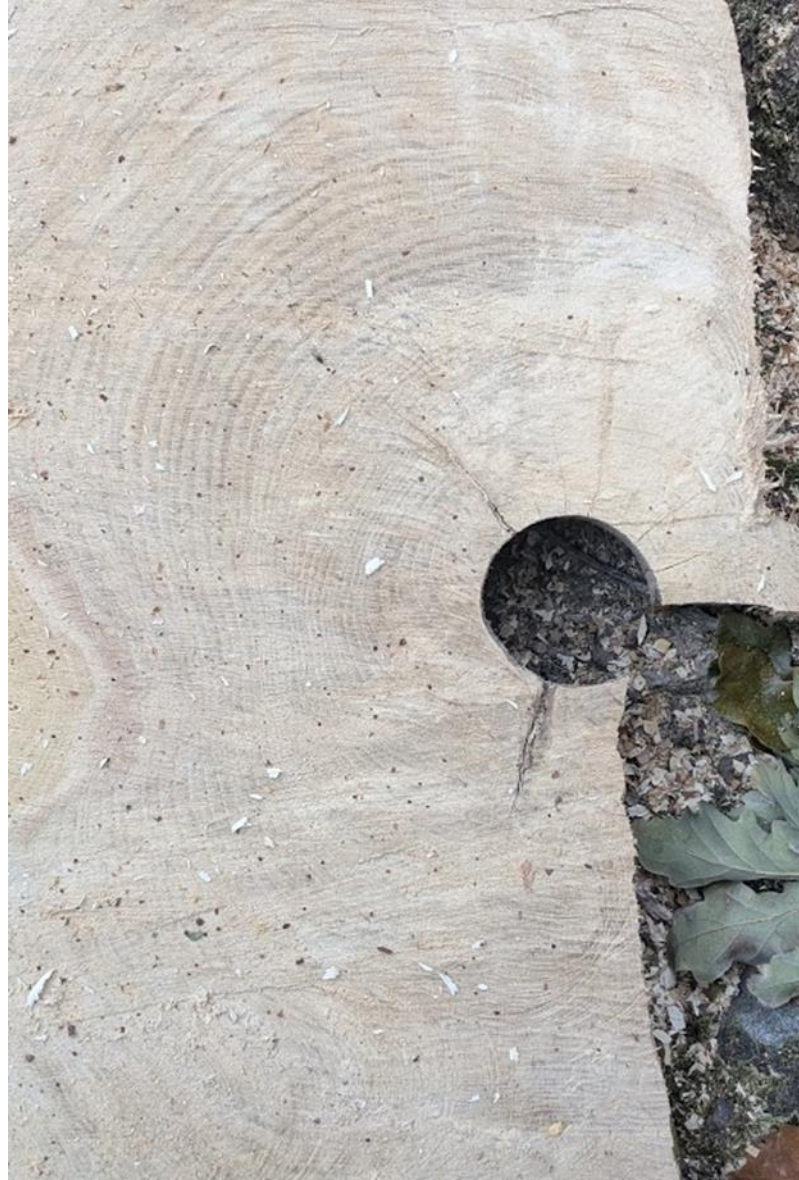
A selection of examples of ring and star shake on the Wyre Forest study site. A large proportion of the trees are afflicted by shake, which compromises the value of the timber. Shake is a major problem facing the land trust who manage the site.
