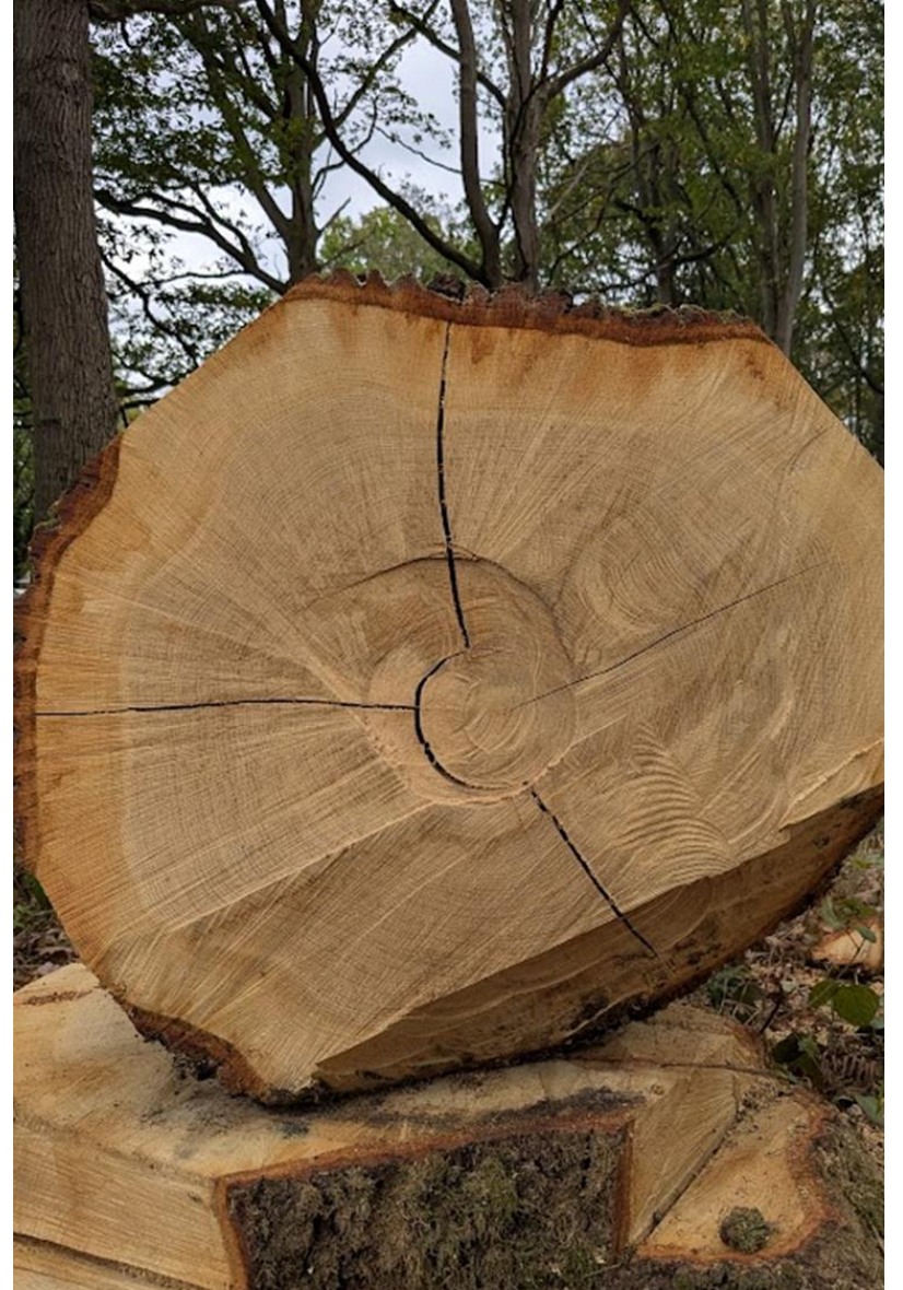
A selection of examples of ring and star shake on the Wyre Forest study site. A large proportion of the trees are afflicted by shake, which compromises the value of the timber. Shake is a major problem facing the land trust who manage the site.
