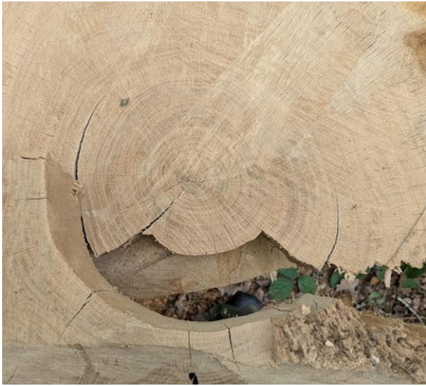
A selection of examples of ring and star shake on the Wyre Forest study site. A large proportion of the trees are afflicted by shake, which compromises the value of the timber. Shake is a major problem facing the land trust who manage the site.
