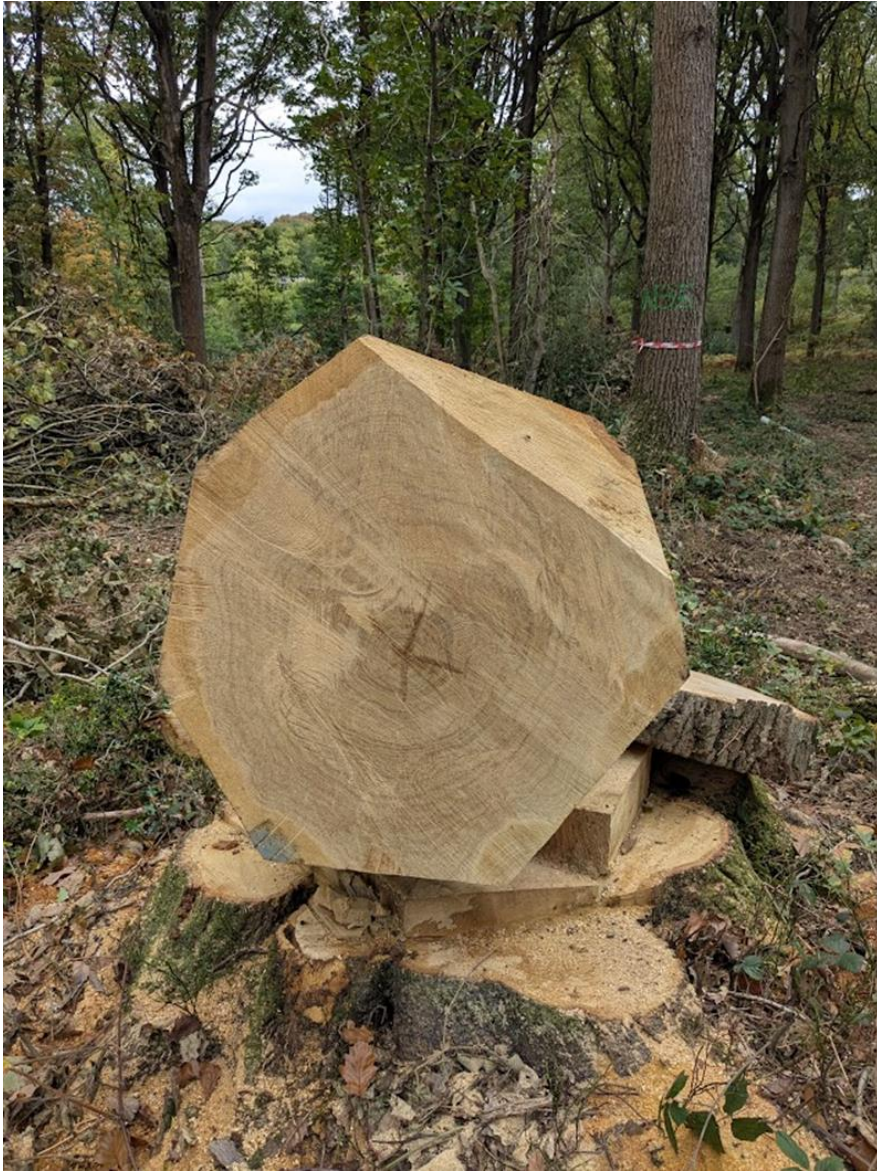
Left: Distinctive star shakes identifiable by the dark staining. Right: Oak stems were presented to us propped up to allow us to inspect the whole section.
